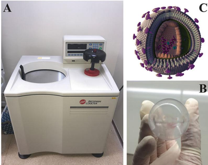
**Fig. 7** Ultracentrifugation procedure following the production process. (a) Ultracentrifugation instrument, (b) viral pellets obtained following ultracentrifugation, and (c) schematic representation of the lentivirus. Image created by Yunus Emre Eksi, MSc
